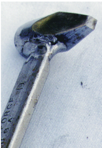
The tip of this drift was broken. Grind the end back flat.
